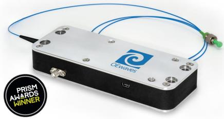
This HI-Q® laser houses a proprietary driver/controller and the OEwaves laser source which is based on a high quality factor (Q) Whispering Gallery Mode (WGM) micro-resonator. The laser is available at a variety of wavelengths in the 780nm region.
