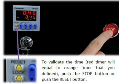
② Push the STOP button to set up the timer
