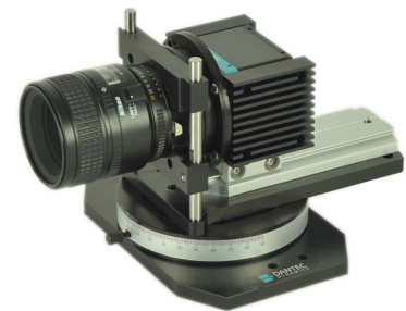
A camera and lens fitted on a Scheimpflug mount.
