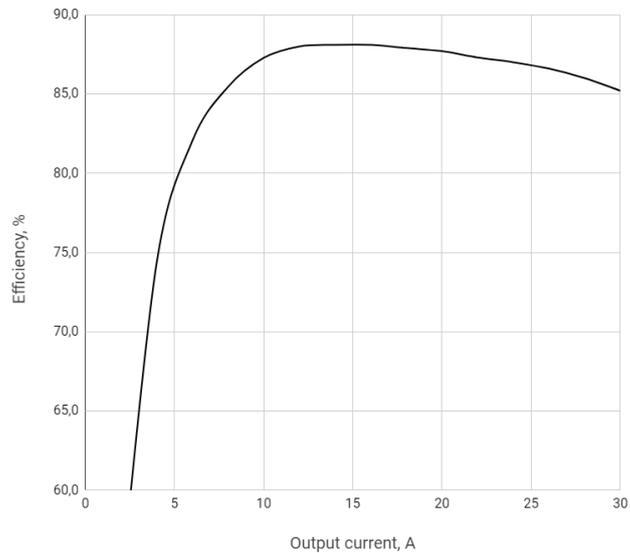
Figure 4 – Efficiency vs. output current at light load
