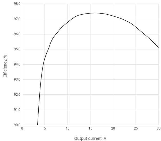
Figure 2 – Efficiency vs. output current at full load
