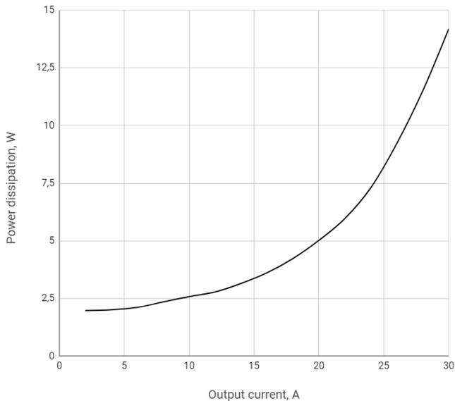
Figure 1 – Power dissipation vs. output current at full load
