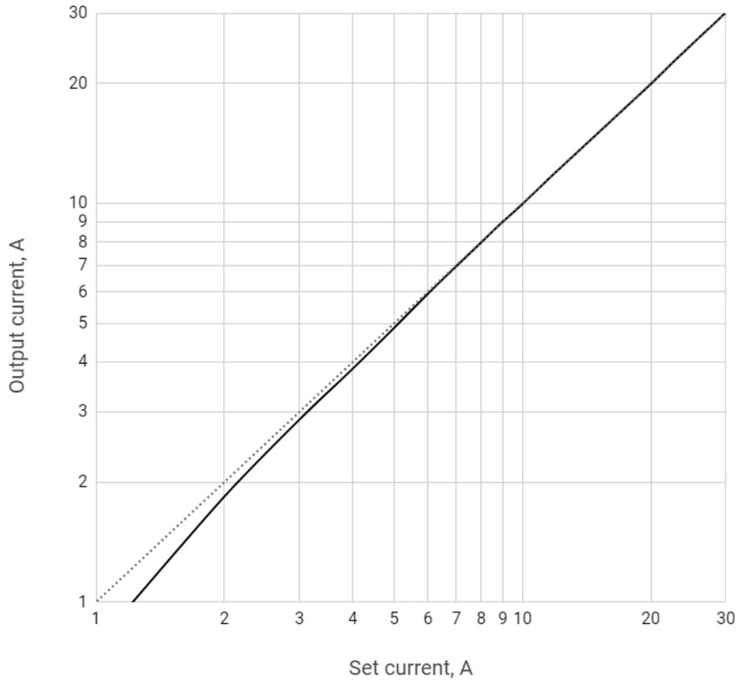
Figure 5 – Regulation characteristic: dotted – ideal, solid – real
