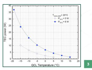
Power consumption of the built-in TEC<sup>1</sup> as a function of the QCL chip temperature for a base plate temperature of  $+20^{\circ}$ C, with and without a thermal load in the QCL.
