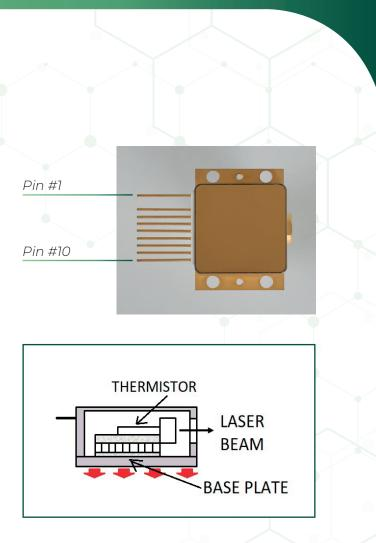
The above HHL-package diagram shows the built-in thermistor that monitors the laser chip temperature. The diagram also shows the base plate that dissipates the heat generated by the TEC and the laser chip.
