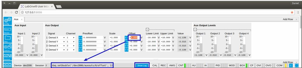
Figure 6.1. When a device's configuration is modified in the LabOne User Interface, the Status Bar displays the equivalent command to perform the same configuration via a LabOne programming interface. Here, the Matlab code to modify auxiliary output 1's offset value is provided. When "Show Log" is clicked the entire configuration history is displayed in a new browser tab.
