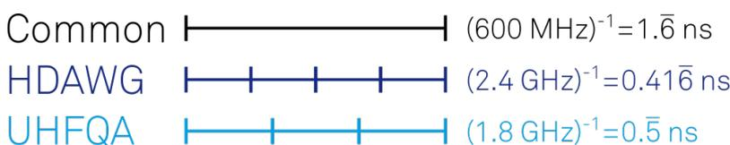
**Figure 3.8. Time alignment of the HDAWG and UHFQA**
