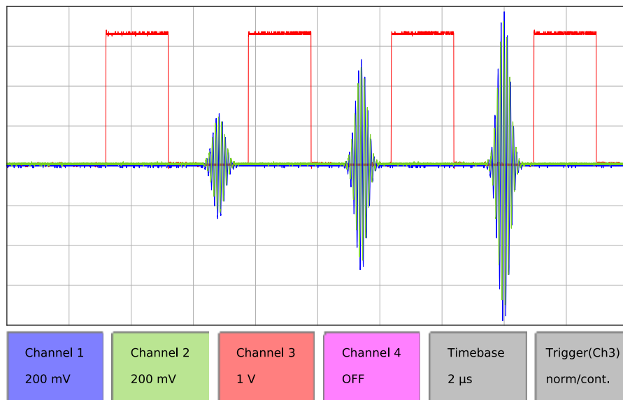
Figure 3.23. HDAWG output signals for a Rabi oscillation measurement as measured with an external oscilloscope
