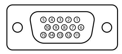
**Figure B.1:** Connector pinout. Relay (-) should be grounded to open the protection relay and enable operation.
