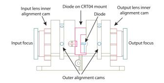
Figure 2.1: Eccentric cam sub-assembly.
