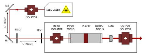
Figure 2.3: Alignment setup for aligning MOA002 to seed laser.
