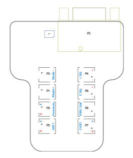
**Figure B.2:** MOGLabs MOA002 laser head board showing connectors for tapered amplifier diode, temperature sensor, TEC and LEDs.
