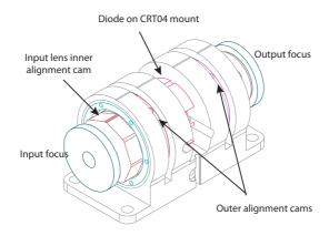
Figure 2.2: Eccentric cam sub-assembly.
