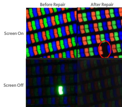
Array repair – block removal
