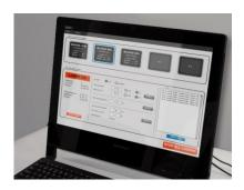
**PC control software -** ML6600 devices are equipped with an external control capability. Together with optional PC software the user controls the laser system via a USB connection. The software enables easy access to control the laser operating parameters such as illumination time, optical output power and input current for the ML6600 laser module.
