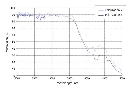
Transmission curve between 2µm and 5µm:
