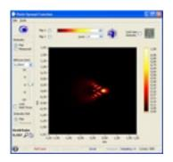
The PSF, or far field, is the spatial dispersion of the energy in the laser's focal plane. It is calculated by combining the phase and intensity measurements on the sensor's surface via propagation of the electromagnetic field in accordance with the law of free space propagation.
