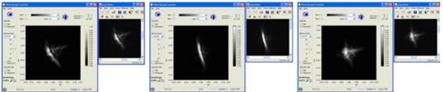
In the 3 screen captures above, taken from actual wavefront measurements performed using HASOv3, you can clearly see that the calculated PSF (larger, left-hand screen capture) is identical to the directly measured PSF (smaller, right-hand screen capture).
