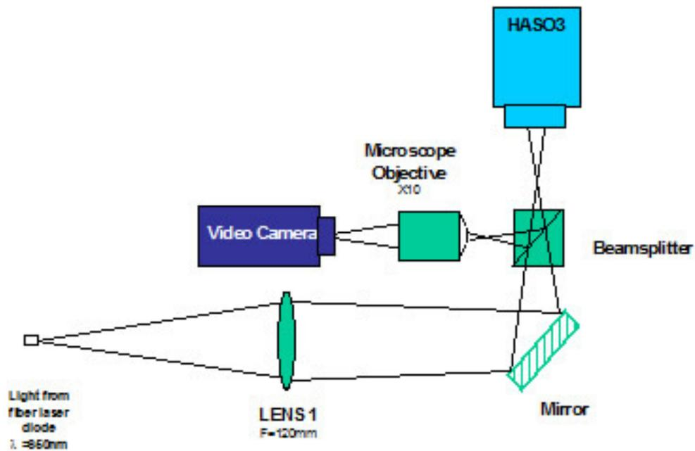
As the screen captures below demonstrate, viewing the results of this test with your HASO™ wavefront sensor on your own is not difficult.
