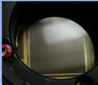
Fig 3. Microlenses and the CCD of HASO wavefront sensor
