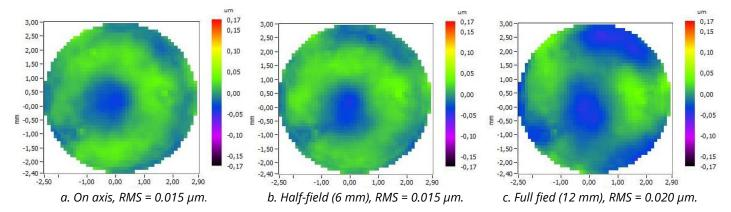
**Figure 13.** Wavefront evolution accros the work field, without the 3<sup>rd</sup> order aberrations influence. The 5<sup>th</sup> order spherical aberration is predominant on axis, but the trefoil prevails at the edge of the work field.
