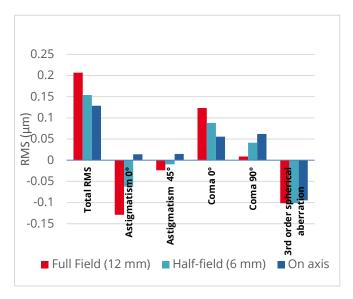
**Figure 11.** Wavefront decomposition over the 3<sup>rd</sup> order aberrations. The presence of Coma in the center of the field points out a centering issue due to one or more optics in the complex lens. Higher order aberrations are negligible compared to 3<sup>rd</sup> order aberrations.
