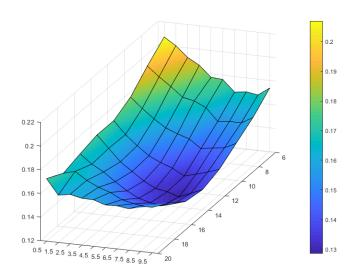
**Figure 10.** Complex lens WFE measurement in the work field. Axes (xOy) stands for the field coordinates, in mm, and the axis (Oz/colormap) stands for the global RMS (Root Mean Square) WFE, in  $\mu$ m.
