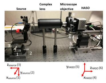
Figure 3. Experimental setup with definition of axes.
