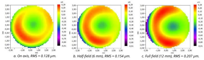
**Figure 12.** Wavefront evolution accros the work field. Coma is significant on axis, which is characteristic of an excentricity defect. Astigmatism appears with the field and prevails at the edge of the field.
