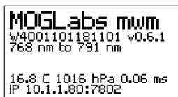
Figure 1.1: Wavemeter on-device display, showing serial number, firmware version, wavelength range, temperature, pressure, exposure duration and IP address.
