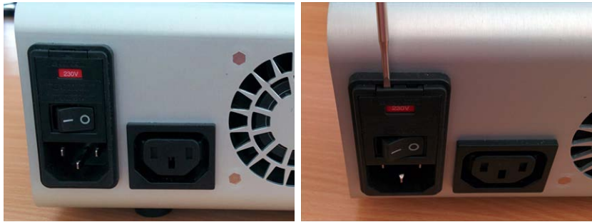
Figure M.2: To change fuse or voltage, open the fuse cartridge cover with a screwdriver inserted into a small slot at the top of the cover, just above the red voltage indicator.
