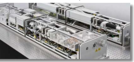
The modular design of the laser head allows a wide variety of resonator configurations and options to be offered, from single rod oscillators to fully birefringence compensating twin-rod-oscillator, twin-rod-amplifier systems. Furthermore, a choice of stable, stable-telescopic or graded reflectivity resonators is available, allowing the customer to specify a system that suits their requirements.
